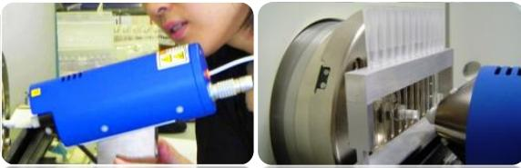
Direct Analysis in Real Time Mass Spectrometry (DART-FTICR-MS)
